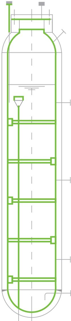
The conversion of ammonium carbamate to urea is a much slower reaction than the formation of ammonium carbamate, and the purpose of the urea reactor is to provide a large space in which the reaction medium will be retained for long enough for it to reach equilibrium. In the conventional CO<sub>2</sub> stripping process some of the ammonium carbamate is first formed in the reactor as well, providing heat to drive the conversion reaction.
