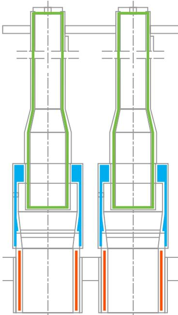
To create a nice falling liquid film down to the heat exchanger tubes there is a sophisticated liquid divider system including the so called liquid dividers. These dividers contain three liquid holes for the liquid distribution and on top a gas restriction for the virgin CO<sub>2</sub>/gas distribution over the heat exchanger tubes.
