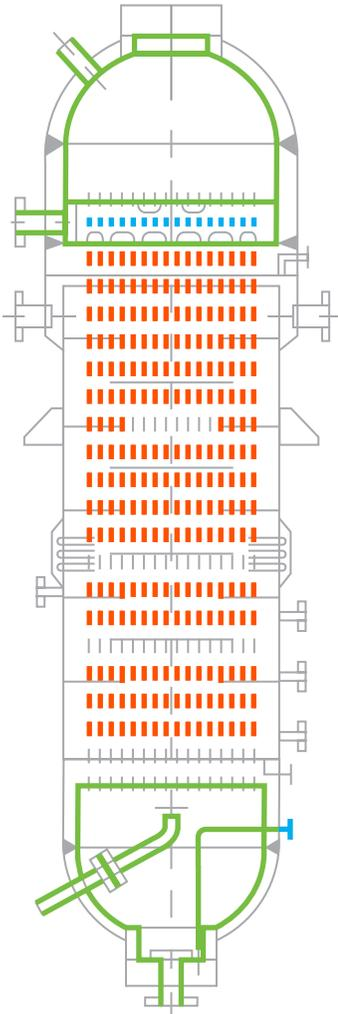
The Safurex® HP STRIPPER is a high pressure carbon steel vessel with a special alloy protection. This stripper is a falling film heat exchanger where liquid is distributed by a liquid distributing system. The liquid divider is based on years of experience and design studies and will be customized according to your process condition.
