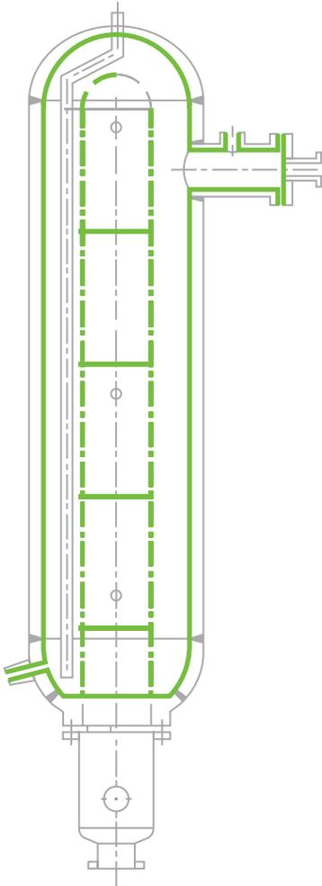
The Safurex® POOL CONDENSER is a submerged high pressure carbon steel vessel with a special alloy protection that has become the industry standard, replacing the falling film type HPCC. To generate the required optimal distribution of gas a special distributor was invented. The distributor including the process baffles and the flow deflector plates creates the most optimal crossflow distribution. The heat is transferred into LP steam by a special designed U-shaped bundle.
